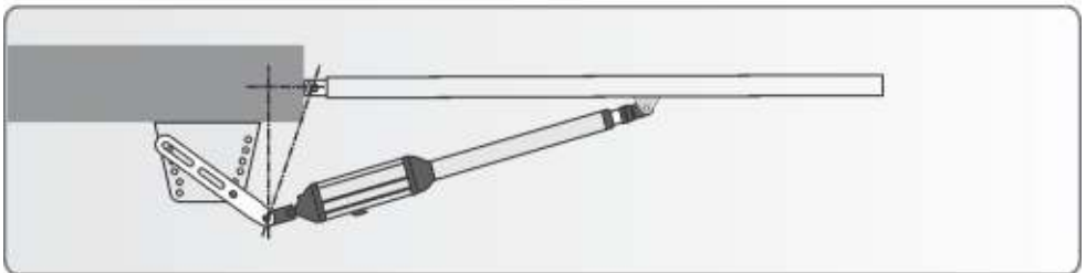
FIGURE 25. INSTALLATION ON A PALISADE FENCE
