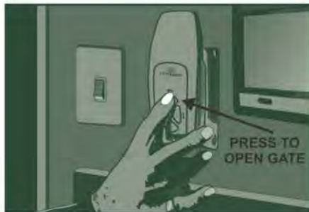
Gate opened from intercom pushbutton inside house.
