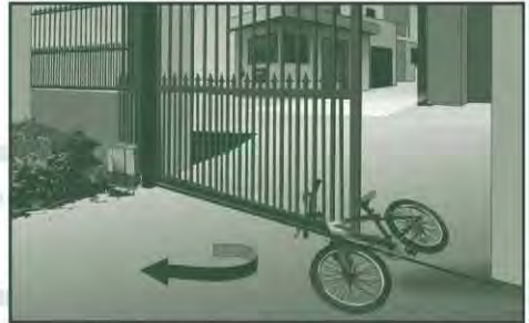
Gate automatically reverses and re-opens
