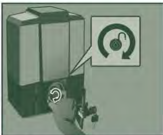
Rotate thumbwheel clockwise until gate is free to move
