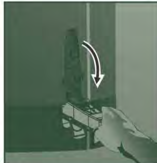
Pull manual release handle down to disengage manual release
