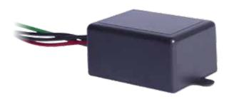
The CP107 is designed to prevent your 12V lead-acid battery from going below 10.6V during a mains power failure. Should the battery voltage drop to 10.6V during a mains power failure, the CP107 automatically disconnects the battery from the load circuitry. Once mains power is restored the battery saver automatically resets, allowing your battery to recharge to full capacity.
