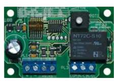
This is a handy timer card, which can be used in many access control applications. A trigger input will latch the output for a variable time.
