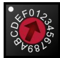
Figure 3 Address switch (SW3) with address 1 selected
