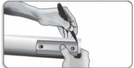
FIGURE 28. MARKING THE POLE
