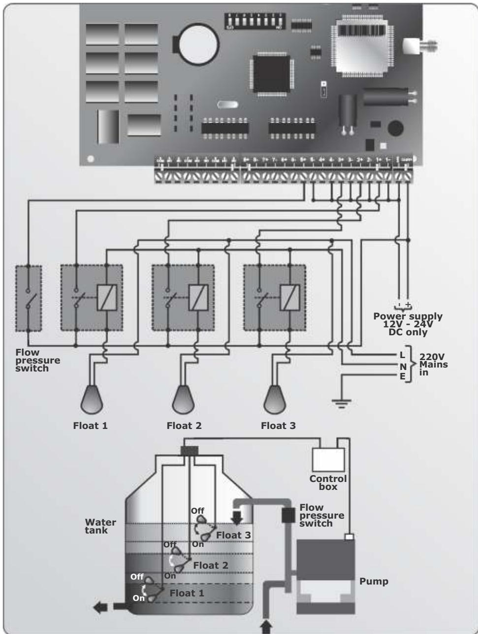
FIGURE 21. MyGSM 8180 CONNECTION TO A WATER TANK WITH 3 FLOAT LEVELS
