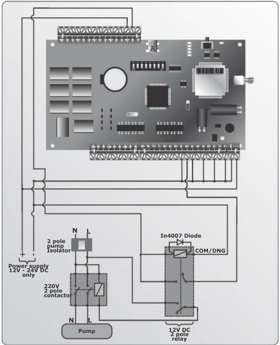
FIGURE 20. MyGSM 8I80 CONNECTION TO A PUMP
