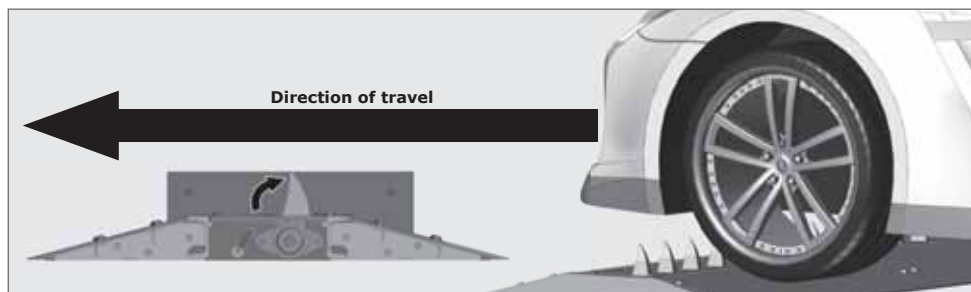
FIGURE 5. SPIKE IMPACT DIRECTION - OPPOSING
