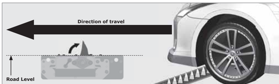
FIGURE 5. SPIKE IMPACT DIRECTION - OPPOSING
