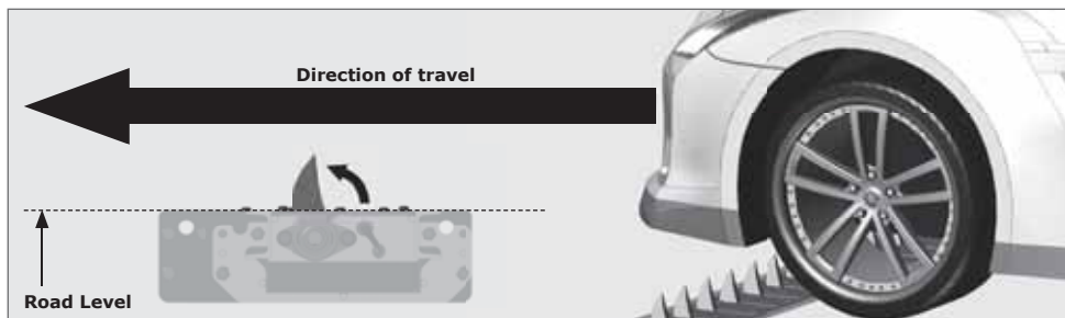
FIGURE 4. SPIKE IMPACT DIRECTION - SIMILAR
