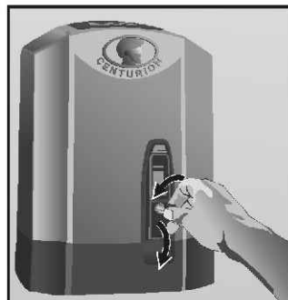
Open lock cover and insert key. Turn key ¼ turn counter clockwise to unlock.
