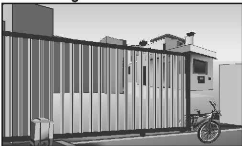
Gate closing into an obstruction
