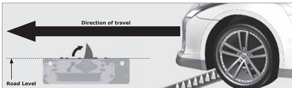
FIGURE 5. SPIKE IMPACT DIRECTION - OPPOSING
