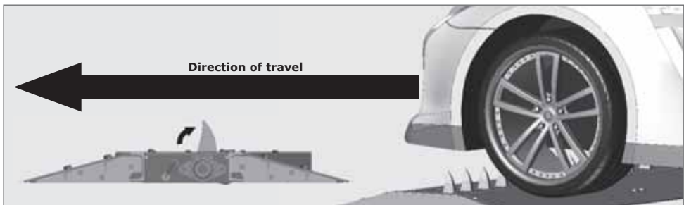
FIGURE 5. SPIKE IMPACT DIRECTION - OPPOSING
