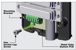
10. Wire your cables to the Wiring Block on the **Metal Gate Station** PCB and fit it back into the **Metal Gate Station** Rear Housing using the inverse movements of step 4.
