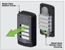
Remove the Metal Gate Station Cover away from the Metal Gate Station Rear Housing.
