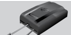
1. Remove the cover from the enclosure using a flat screwdriver.
