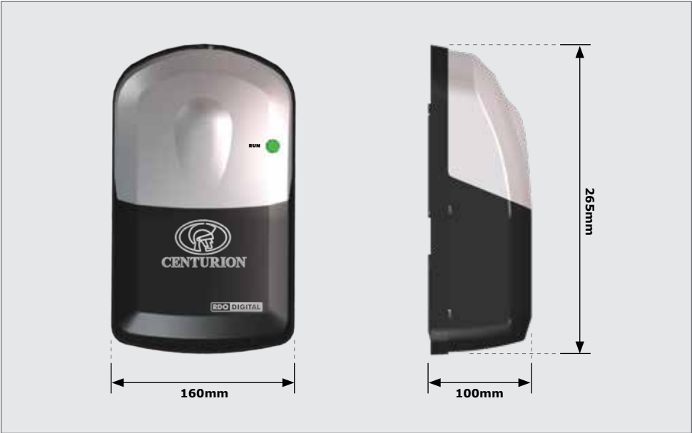
FIGURE 2. RDO DIGITAL CONTROL BOX PHYSICAL DIMENSIONS
