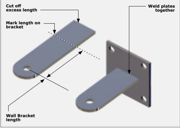
FIGURE 32. CUT AND WELD WALL BRACKET
