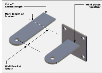
FIGURE 20. CUT AND WELD WALL BRACKET
