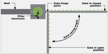
FIGURE 9. PILLAR HINGE DEPTH LIMITATION FOR 90° INWARD-OPENING GATE
