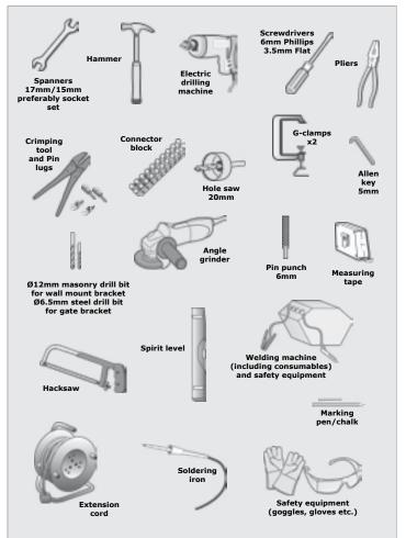
FIGURE 6. REQUIRED TOOLS AND EQUIPMENT
