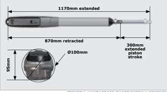
FIGURE 1. VANTAGE 300 SMART OVERALL DIMENSIONS
