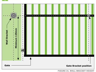
Mark the calculated length required on the Wall Bracket.
