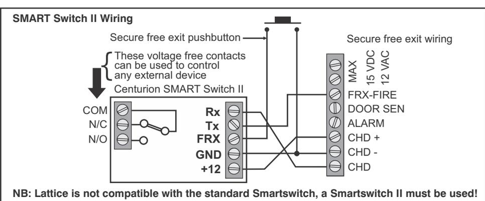
Fig 5 Connection to Centurion SMART Switch II
