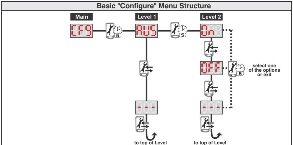
Fig 20 Basic "Configure" Menu Structure
