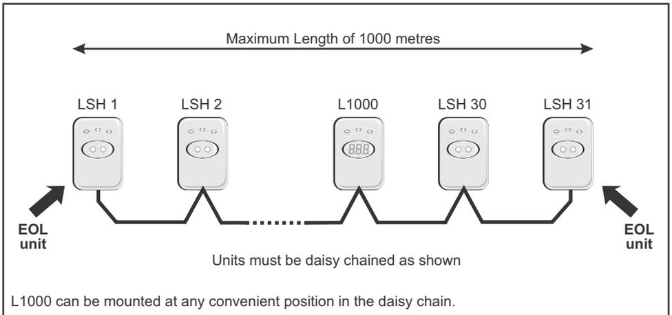
Fig 11 Sketch showing daisy chaining of connected units
