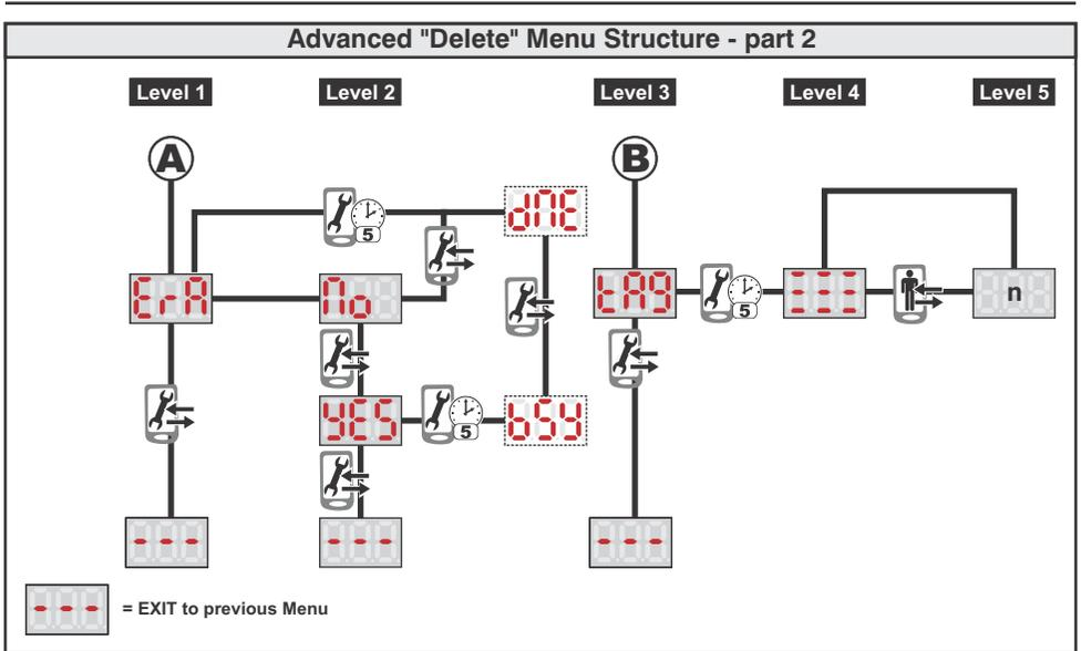
Fig 24 Part 2 of Advanced "Delete" Structure
