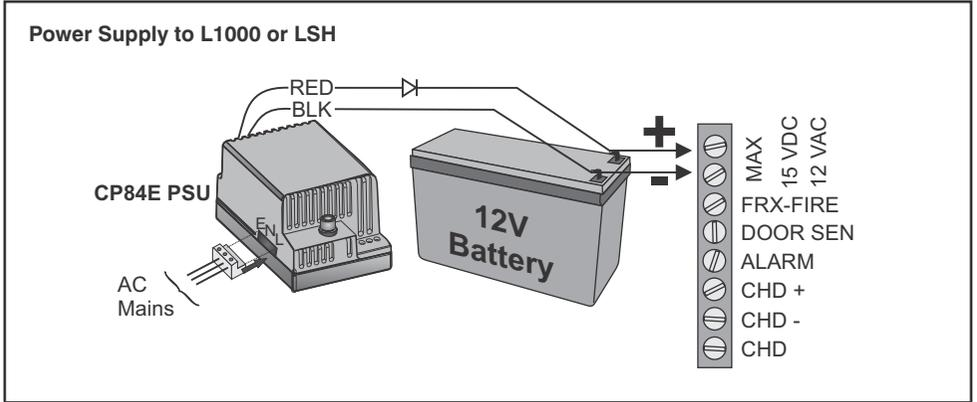
Fig 3 Power Supply to L1000 or LSH
