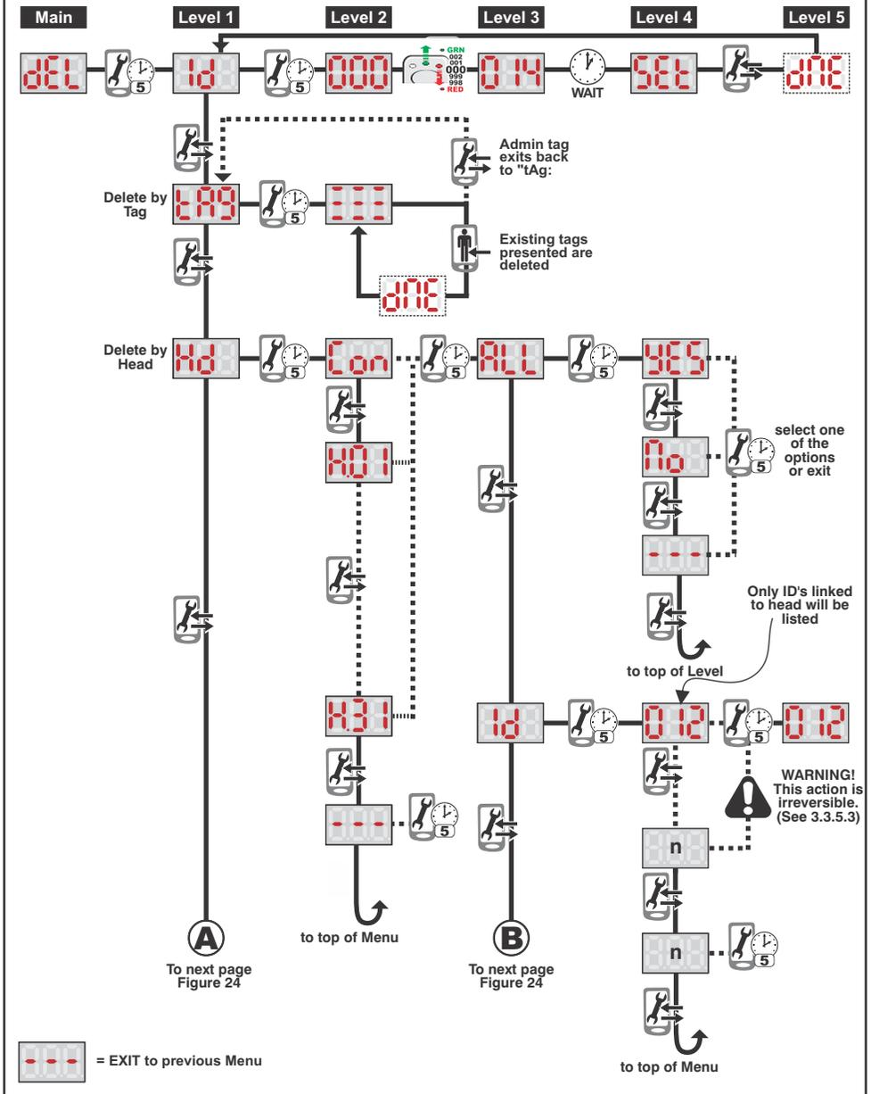
Fig 23 Part 1 of Advanced "Delete" Structure
