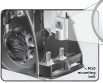
Screw the Theft-resistant Locking Nut onto the M10 mounting nut. With the standard mounting nut in place, the **Theft-resistant Locking Nut** is screwed onto the right M10 mounting bolt, located closest to the gate, by hand as far as is possible so that the hole for the padlock is facing you as shown in the image. Lock the 60mm discus lock onto this nut.
