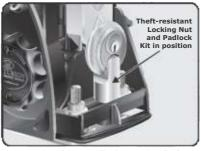
Insert the Discus padlock onto the Theftresistant Locking Nut and lock. When using this specific bolt position as well as the supplied 60mm discus lock, the **Theftresistant Locking Nut** and **Discus Padlock** Kit cannot be removed without seriously damaging the gearbox, or destroying the padlock, as the wall on the gearbox interferes with the rotation of the nut with the lock in place.
