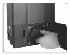
Ensure that the gearbox is engaged by turning the thumbwheel anti-clockwise before fitting the **Thumbwheel Guard**. It must not be possible to move the gate by hand.
