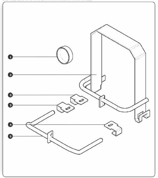
FIGURE 1. THUMBWHEEL GUARD AND THEFT-RESISTANT CAGE PARTS IDENTIFICATION
