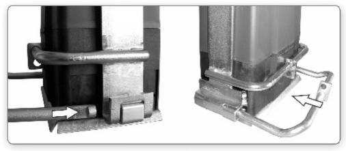
7. Fit the front bar to the assembly by feeding both legs of the bar through the bracket and overstrap.
