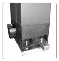
2. Remove side vents, retaining nuts and washers. Fit a bracket to each of the left hand side retaining studs.
