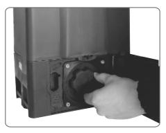
Ensure that the gearbox is engaged by turning the thumbwheel anti-clockwise before fitting the **Thumbwheel Guard**. It must not be possible to move the gate by hand.
