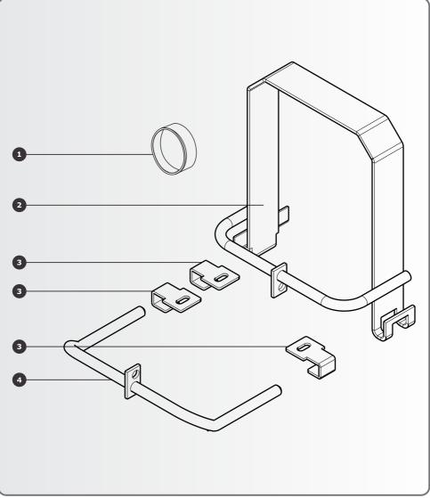
FIGURE 1. THUMBWHEEL GUARD AND THEFT-RESISTANT CAGE PARTS IDENTIFICATION
