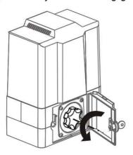
ROTATE THUMBWHEEL ANTI - CLOCKWISE TO RE - ENGAGE
