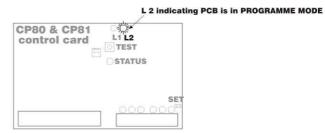
STEP 2 Hold TEST P/B DOWN until number of flashes of LED, L1, corresponds to the TIMER to be selected as shown in TABLE 6.1, then release P/B.
