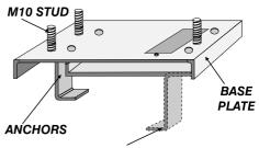
BEND THE ANCHORS VERTICALY TO FIX THE FOUNDATION PLATE INTO THE CONCRETE
