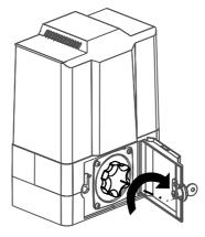
ROTATE MANUAL DISCONNECT THUMBWHEEL CLOCKWISE UNTIL GATE IS RELEASED.
