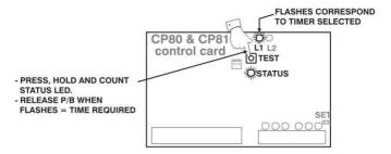
L 1 will extinguish & L 2 will illuminate allowing selection of more timers or functions. ( See Procedure 4 or 5 ).
