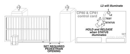
NOTE: 'STEP 5' MUST BE PERFORMED EVEN IF THE PEDESTRIAN FACILITY IS NOT USED.
