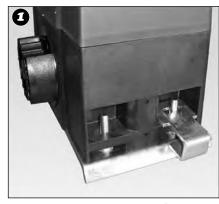
Remove side vents, retaining nuts & washers. Fit a bracket to each of the LHS retaining studs.
