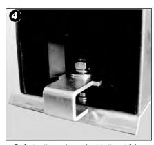
Re-fasten the washer and nut to the retaining stud to secure the bracket.
