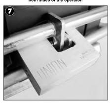
With the front bar fully engaged with the overstrap, secure the assembly by locking a good quality padlock through the aligned barrel holes on the overstrap and front bar.
