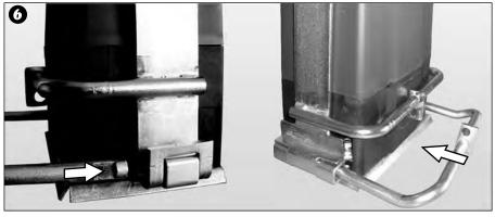
Fit the front bar to the assembly by feeding both legs of the bar through the bracket and overstrap.
