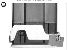
Finally, secure the cage by locking the front strap and the overstrap together with a padlock with substantial shackle, sized such that minimum shackle is exposed.
