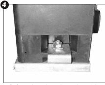
Re-fasten the washer and nut to the retaining stud to secure the bracket.
