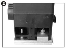
Re-fasten the washers and nuts to the retaining studs to secure the brackets.
