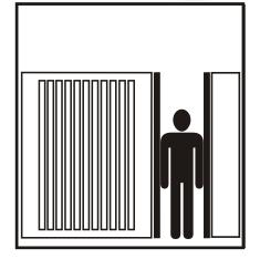
It has become the modus operandi of would-be intruders to hold open an entrance gate by covering up the system infrared safety beams.
