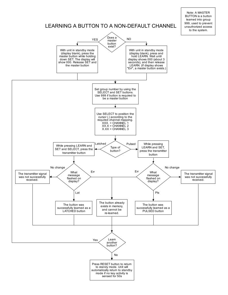
Note: A MASTER BUTTON is a button learned into group 999, used to prevent unauthorized access to the system.
